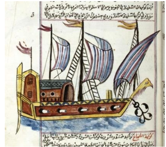
Paris BN Arabe 2178 1762-63 AD Qazwini n.b. – bird's head on bow; anchor, ladders external tiller
